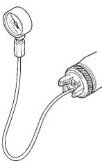
The purpose of this test kit is to measure air cap atomizing air pressure at the center air port of the air cap. Used to confirm code compliance and as a daily quality control measure.
