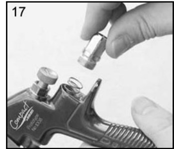
17. Replace Valve Spring and screw in Housing (10).
