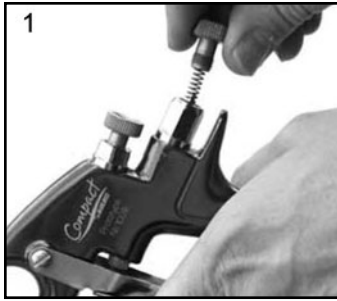
1. Remove Adjusting Knob (7), Spring (8), and Needle (9).
