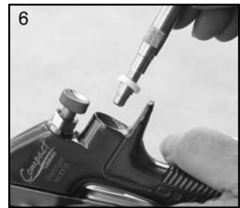
6. Remove Valve Seat.
