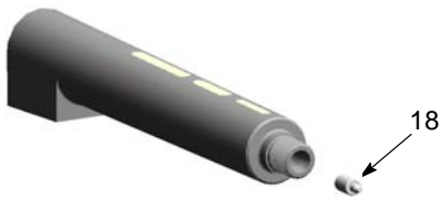
Figure 27 Removing the Contact Spacer
