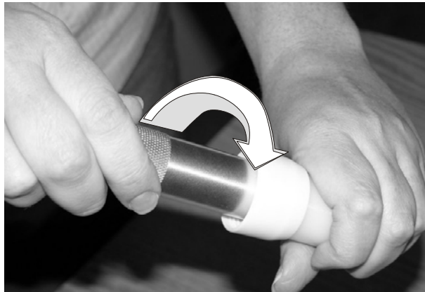
Figure 5 Nozzle Disassembly Step 2A
