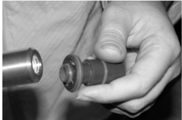
Figure 7 Nozzle Disassembly Step 3 (New Style Shown)
