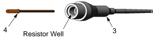
Figure 25 Removing the Resistor from the Holder
