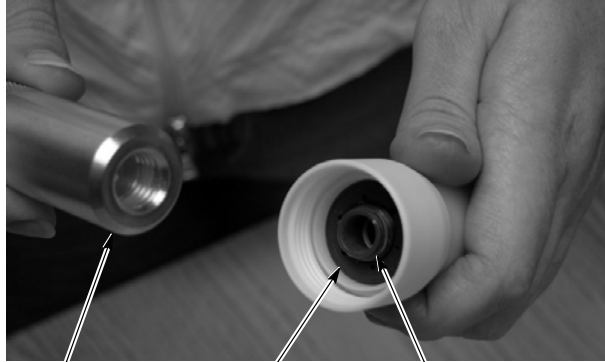
Figure 4 Nozzle Disassembly Step 1 (Shown with Nut Installed)
