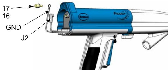
Figure 19 Disconnecting the Control Cable
