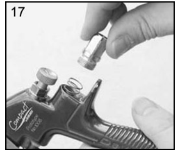
17. Replace Valve Spring and screw in Housing (10).
