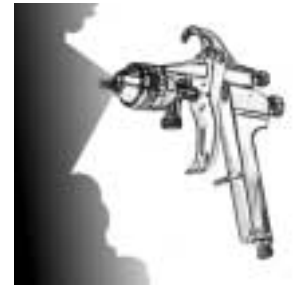
Conventional High Pressure Spray Gun Overspray
