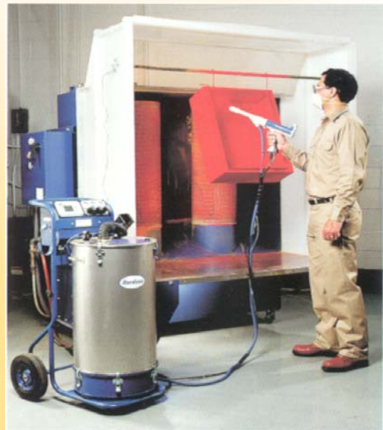
Sure Coat Manual Spray System with Portable Hopper Feed
