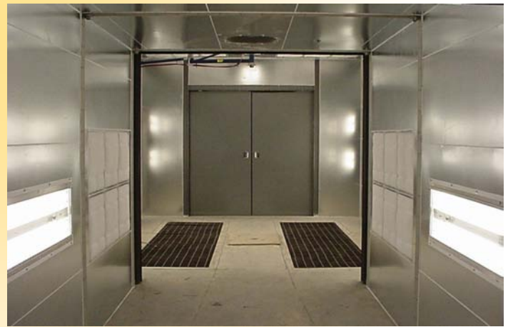
Down draft booth with doors at both ends and a ceiling mounted boom to keep hose lines off the floor
