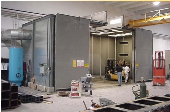
Blast booth with rubber lined walls, crane slot, centrifugal fan and dust collection module
