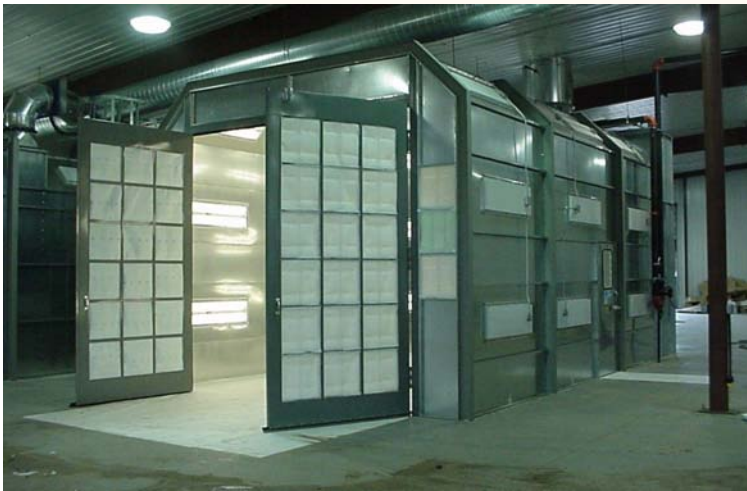
Drive through cross-draft spray booth
